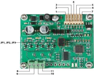
The three jumpers JP1, JP2 and JP3 can be set in the configuration as per the below table to provide a physical slave address to the drive. In the below table a value of '0' corresponds to a state where the jumper is not connected and a value of '1' corresponds to a state where the jumper is connected. If none of the jumpers are connected the drive has been programmed to use the Slave ID 1 in default mode which can be changed from 1 to 247 using Modbus commands.
