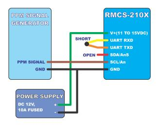
To enable the PPM signal input to the RMCS-210x the UART TXD and UART RXD lines of the RMCS-210x must be shorted together. Remember to power – off and power – on RMCS-210x after shorting RXD and TXD.
